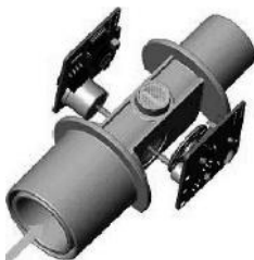
Figure 7. PHASEIN IRMA IR light path through the IRMA airway adapter.
