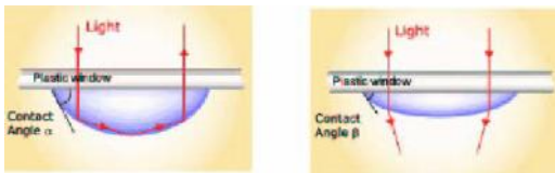
Figure 10. Effect of condensed water on light transmission.
