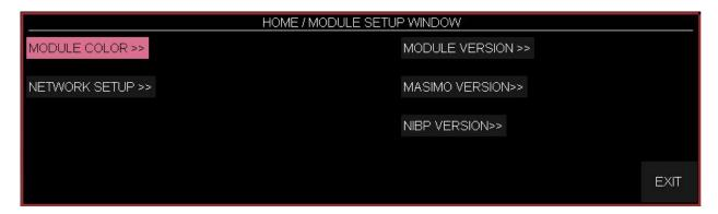
Pick "MODULE COLOR" in MODULE SETUP window to call up the following window. You can set color of all parameters except ECG in this window. Select <DEFAULT COLOR> to restore default color of all modules as shown in the below figure.
