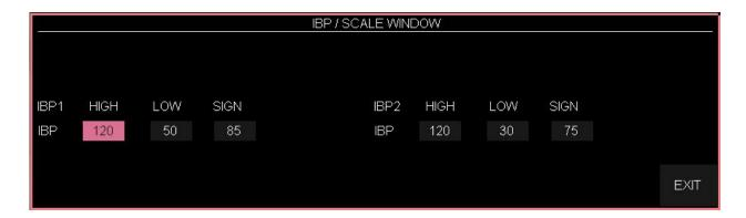
The waveform and corresponding scale appears in the IBP waveform area with 3 dotted lines representing HIGH limit scale, SIGN cursor, and LOW limit scale from the top to the bottom that values of the three scales can be manually set or automatically by Auto scale. You can change the high and low scales for IBP, ART and LVP labels by step of 10 and for PAP, RVP, CVP, ICP, LAP and RAP labels by step of 5. The cursor changes by step of 1 for all labels.
