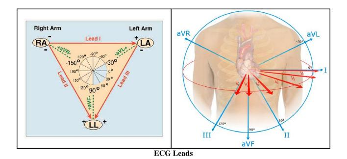
Depending on cable's type (3-WIRE or 5-WIRE), you can choose different leads I, II, III, aVR, aVL, aVF and V.
