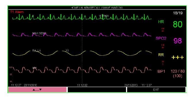
The time of alarm occurrence is displayed by a vertical dotted line. The signals of 5 seconds before and after this time are displayed in the window.
