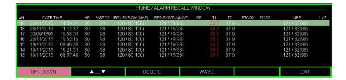
Alarm data including the number of alarm event, date, time and HR, SpO2, IBP1-SYS/DIA (MAP), IBP2-SYS/DIA (MAP), PR, T1, T2, ETCo2, FICo2 and NIBP values as well as page number are displayed in this window.
