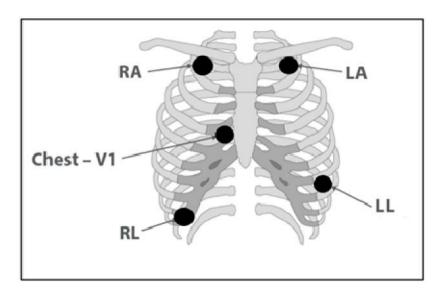
**Electrode's locations for 5-wire ECG Cable**
