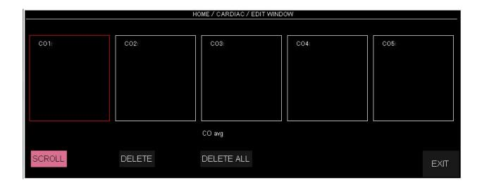
Numeric value, curve and time of the last five C.O. measurements are displayed in this window. Averaged C.O. value is displayed below the window. User can identify and delete erroneous measurements and then average value of other measurements will be recalculated by the system.
