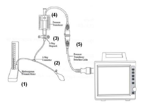
Mercury calibration should be performed by the biomedical engineering department either whenever a new transducer is used, or when system accuracy is in doubt.
