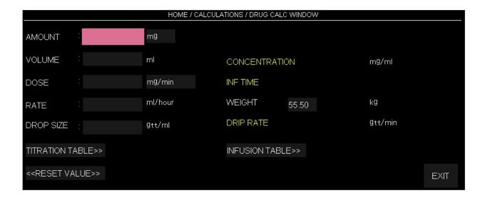
This window is used to calculate rate, dosage, amount or volume, capacity and time of drug infusion. Infusion rate based on Drop Size is defined as Drip Rate.
