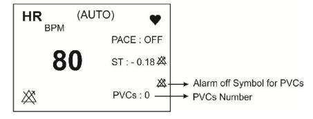
Figure 14-1 PVC value in ECG parameters area
