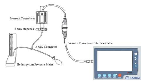
Figure 3-44 calibration equipment connection
