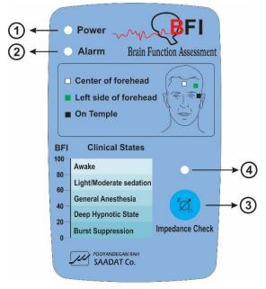
Figure 3-73 BFA module keys and indicators
