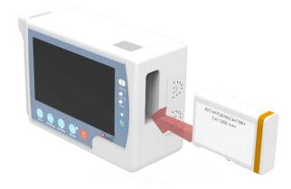
To remove the battery, press the battery eject button (figure 1-9 a). When the battery is released, you can remove it from the compartment.
