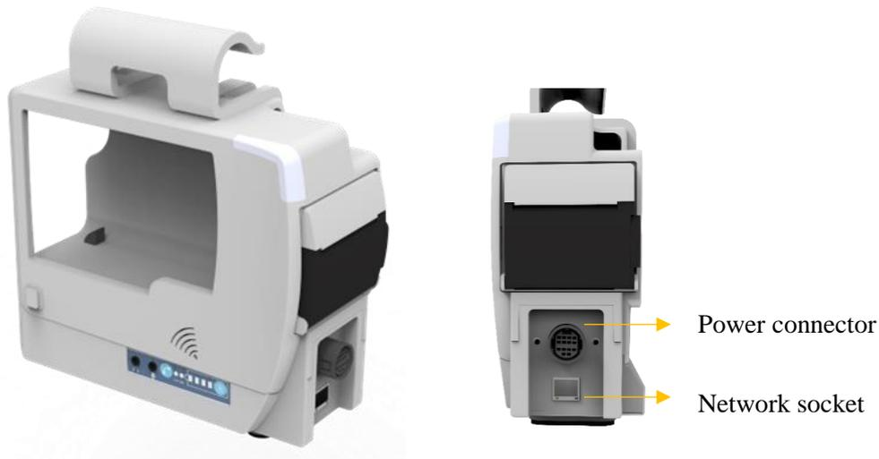
Figure 1-6 TC station and its connectors
