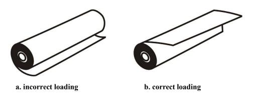
Figure 16-3 Recorder paper loading
