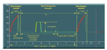
Figure 8-4- Pressure curve in V-SIMV mode
