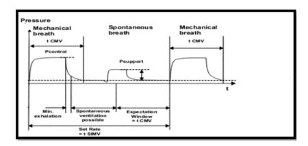
Figure 8-5- Pressure curve in P-SIMV mode
