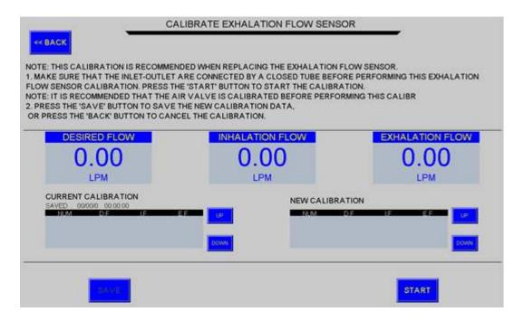
Figure 7-4 Exh Flow Sensor Calibration page
