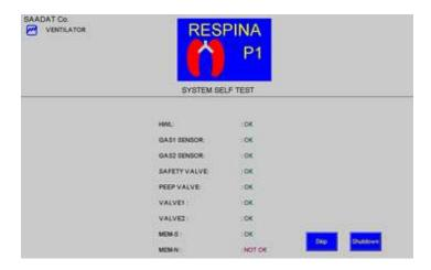
Figure 5-2 memory failure
