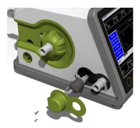
Loosen the screw of the oxygen sensor cover and remove the cover. Carefully remove the oxygen sensor and replace it with a correct one. Make sure that the oxygen sensor cable is connected securely.
