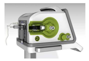
Carefully remove the exhalation flow sensor and replace it with a correct one. Connect the flow sensor cable securely.
