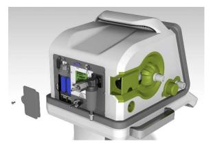
Remove the battery and replace it with a correct one.
