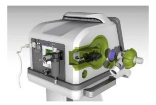
Remove the exhalation valve, exhalation valve- flow sensor interface and the membrane.
