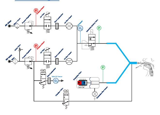
Figure 10-1 Pneumatic diagram
