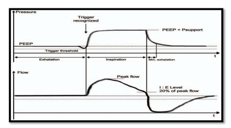
Figure 8-6- Pressure and flow curve in PSV mode
