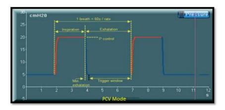
Figure 8-3- Pressure curve in PCV mode
