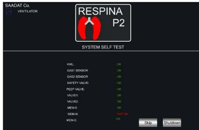
Figure 5-2 memory failure
