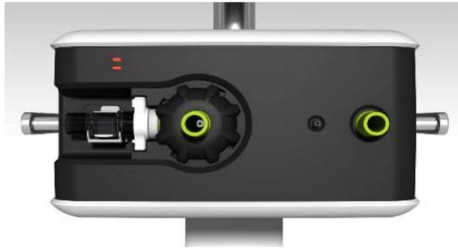
Detach the exhalation flow sensor from exhalation valve.
