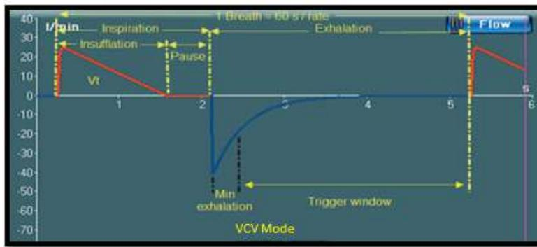
Figure 8-1- Flow versus time curve in VCV mode
