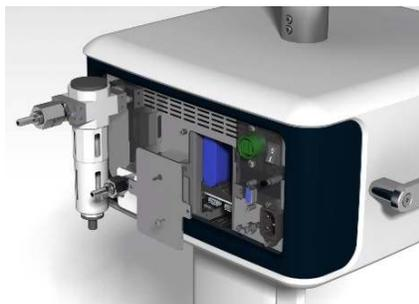
Remove the battery and replace it with a correct one.
