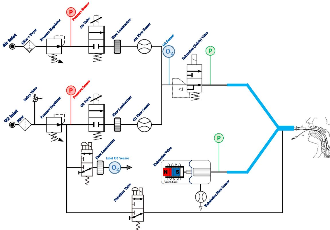
Figure 10-1 Pneumatic diagram
