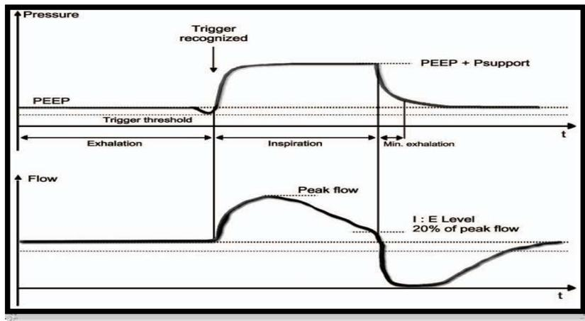
Figure 8-6- Pressure and flow curve in PSV/CPAP mode
