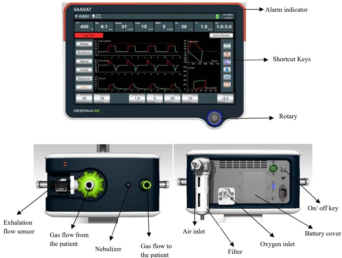
Figure 2-1 Different parts of ventilator
