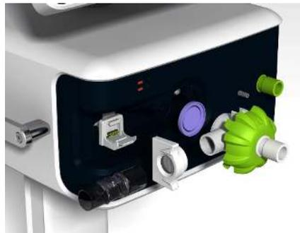
Remove the exhalation valve, exhalation valve- flow sensor interface and the membrane.
