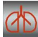
Press this icon on the right-side menu of the ventilator to deliver one breath to patient in the current setting. In this condition "Manual" is displayed on the screen. In A/C and APRV modes the manual inspiration is mandatory and in PSV and VSV modes the manual inspiration is an assisted breath. In SIMV modes the manual inspiration could be mandatory or assisted breath depending on maneuver. The manual maneuver is active in all ventilation modes.
