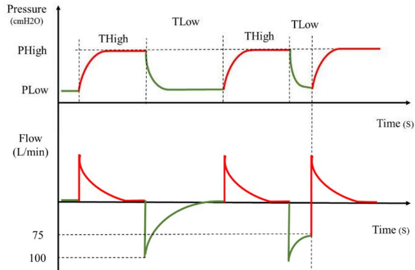
Figure 8-7- Pressure and flow curves in APRV mode with adjustable Auto Flow
